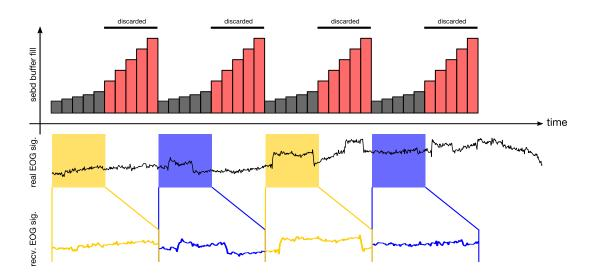
Figure A.2: Signal corruption due to too low packet reception speed. The EOG signal is only partially received and scaled to fill the gaps.
