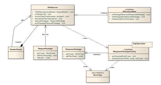
Figure 3.2: TMSi protocol stack architecture
