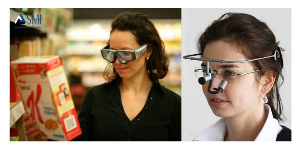
Figure 2.1: SMI Eye Tracking Glasses (courtesy SensoMotoric Instruments GmbH, Dikablis (courtesy Ergoneers GmbH)
