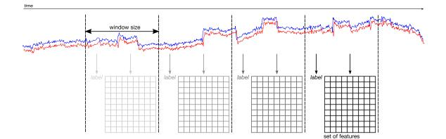
**Figure 5.1:** The data is segmented into windows of 15,10 and 5 minutes. For each window a set of features is computed. Those features include mean blink length and rate, mean fixation length and rate and saccade amplitudes. In addition to the features, each window is assigned a label using majority vote.
