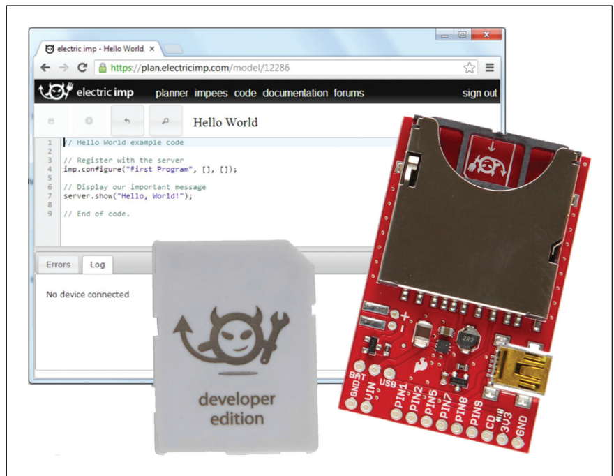
Figure 2. Electric Imp's Web-based editor (background), the SD card form factor main board (center), and the Sparkfun breakout board (right). Written Squirrel code is automatically compiled in the cloud and the binaries are deployed seamlessly to the device over the Internet.
