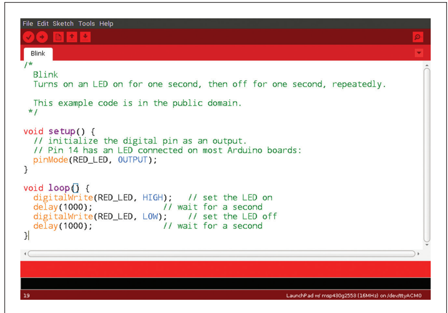
Figure 1. The Energia integrated development environment (IDE) provides a similar development experience to the Arduino IDE. It is based on the Wiring and Arduino framework.
