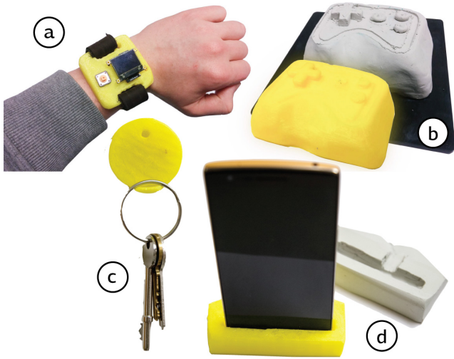
Figure 9. Objects designed with ReForm. (a) User wearing the exported smartwatch prototype. (b) 3D printed and clay versions of the game-controller. (c) Key hook. (d) Phone dock and corresponding clay object.
