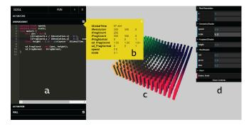
**Figure 1:** The SDSL IDE. (a) The arrangement, actuation and pixel shader editors. (b) The realtime program inspector. (c) Program running in the simulator. (d) Uniform control panel.
