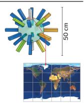
Figure 4: Different geometry shader applications. (left) mapping a physical actuator arrangement to the pixel space of a camera image. (right) Unwrapping a spherical actuator arrangement to a flat texture space.
