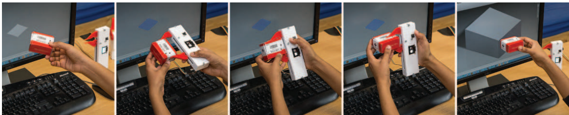
Fig. 4.4 Creating a box (from left to right): select the ground plane, measure width, height and depth.
