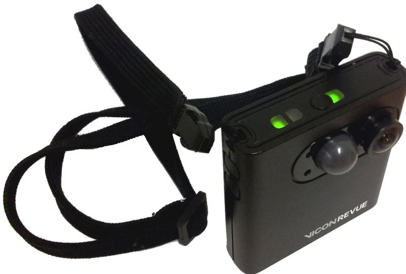
**Figure 3.8:** Vicon REVUE, a commercial version of the Microsoft SenseCam
