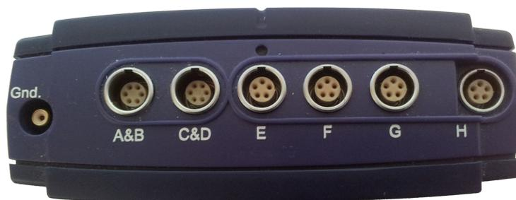
**Figure 3.4:** Top side of the Mobi providing the female electrode ports
