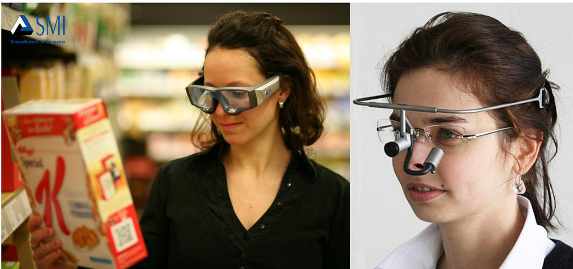
**Figure 2.1:** SMI Eye Tracking Glasses (courtesy SensoMotoric Instruments GmbH, Dikablis (courtesy Ergoneers GmbH)
