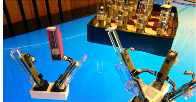
Figure 1: ShapeClip in 4 different configurations deployed on a Microsoft SUR40.
